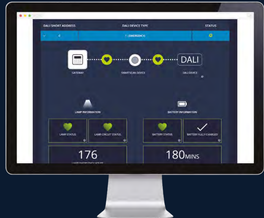
SmartScan Emergency Status Reporting
