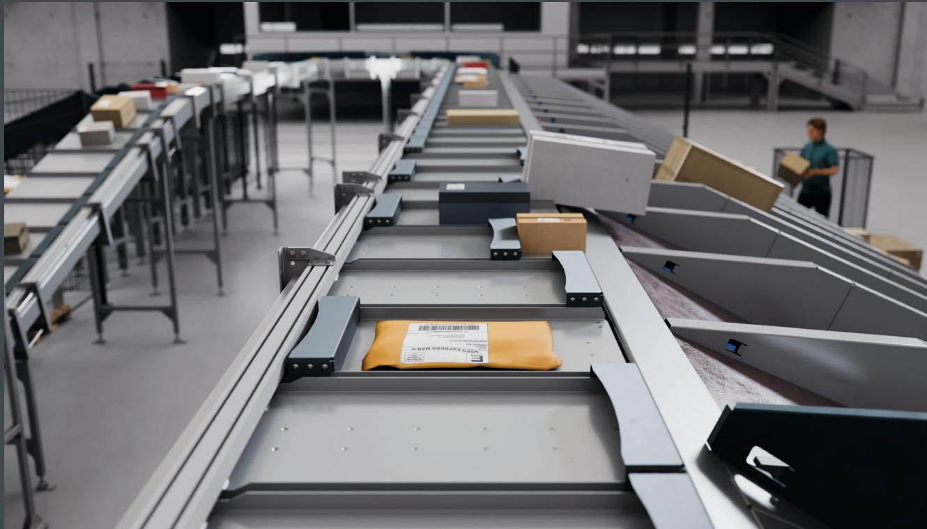
The GEBHARDT Push-Tray Sorter is an innovative automated sorting system specifically designed for logistics and dispatch centres. With remarkable precision and speed, it ensures the smooth sorting and distribution of a wide range of products. Its flexibility allows the Push-Tray Sorter to handle items of various shapes and sizes, making it an ideal solution for companies with diverse product portfolios.
