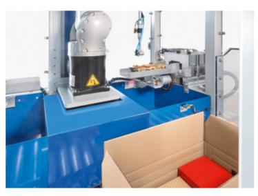
2. PRODUCTION AND PROVISION OF THE PROTECTIVE PACKAGING MATERIAL IN THE REQUIRED LENGTH AND WIDTH.
