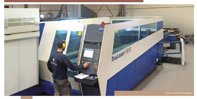
Some of our machines are equipped with a bevel head for making interior and exterior chamfered edges
