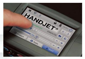
The touch screen can be used to create and edit print messages as well as adjusting print settings including print density and size. Message storage is virtually unlimited with folder-based organisation.
