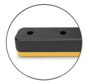
The twin layered Monoplex product offers a softer upper layer which dissipates energy whilst the lower harder layer provides rigidity around the fixing holes. This ensures the StepBumper remains strong under impact and distributes energy across the product, reducing the risk of damage and minimizes the risk of fixings pulling out of the ground.
