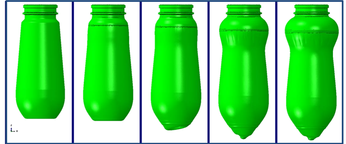
Illustration: simulation of the resistance of PET aerosol to extreme high temperature Aerosol initially filled with appropriate gas at nominal pressure
