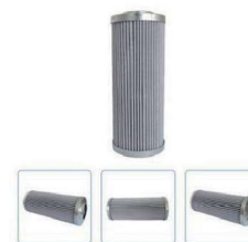
Model: 0240D Size: \Phi 69 \times \Phi 34.2 \times 173 mm Filtering accuracy: 10\mu\text{m}
