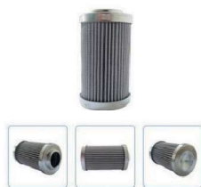
Model: 0060D Size: \Phi 47 \times \Phi 22.5 \times 84 mm Filtering accuracy: 10\mu\text{m}
