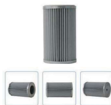
Model: G1.5 Size: \Phi 120 \times \Phi 69 \times 210 mm Filtering accuracy: 50 \mu m
