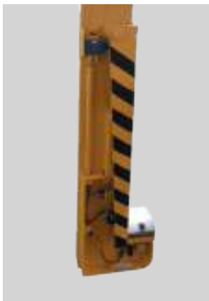
PENDULUM with limit switch for closure stop
