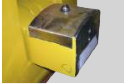
ANTI-OPENING SENSOR Installed on foot of grip
