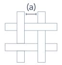
APERTURE SIZES Our standard filter cloths range from 2,000 micron to 3 micron aperture, the measurement being made across the square between the insides of adjacent threads, as shown.
