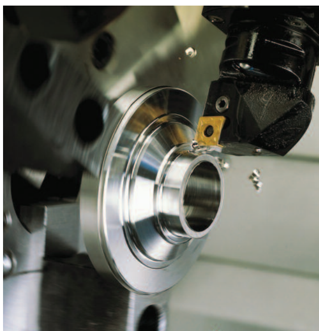
Figure 3. Sanmac 2205 offers 'enhanced machinability as standard' with improved chip-breaking properties.
