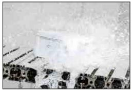
Water and contact protection testing IPx6 / IPx7 / IPx8 / IPx9.
