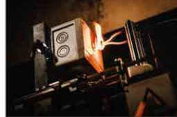
**Glow wire resistance, climatic chamber** And many more tests.
