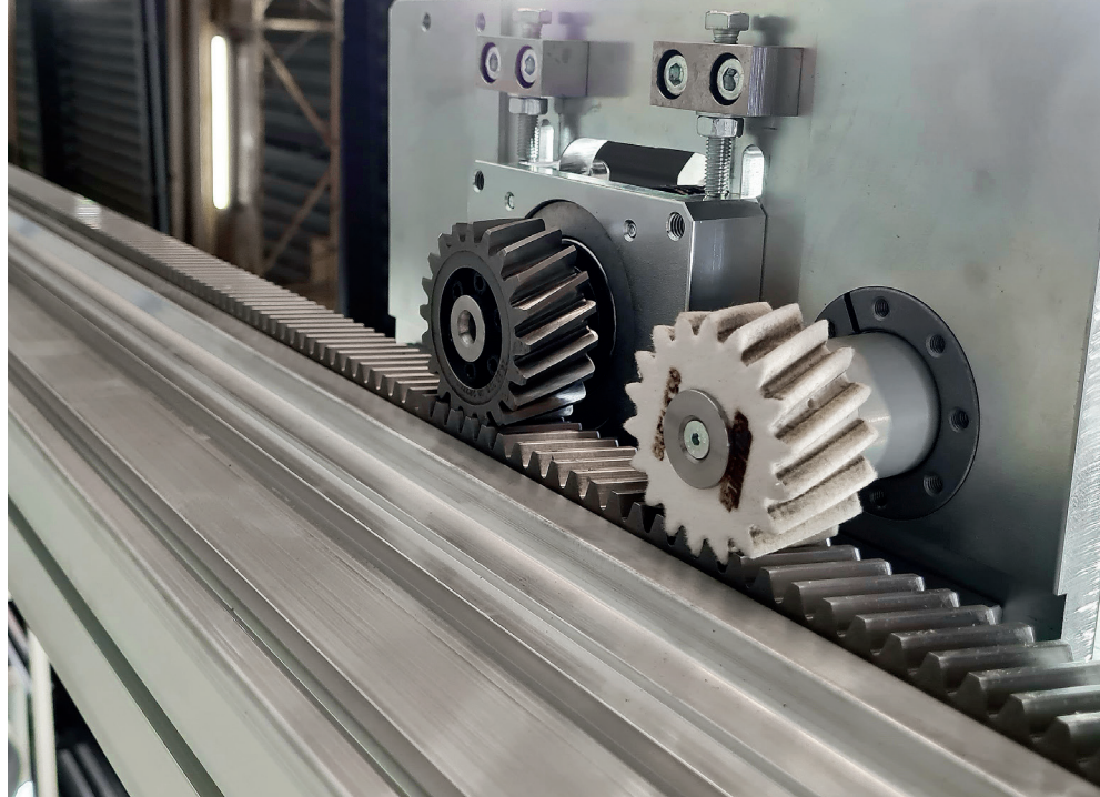
Picture description: The rack and pinion drive of a portal machine is lubricated with an ATLANTA felt gear.
