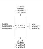
Small distribution board - Industrial Quality -, 2-row, 28 distribution units, 150 mm rail spacing, integrated ventilation elements to reduce the formation of condensate water, elastic entries on top, masking and labelling strips, additional double-membrane seals and other accessories
