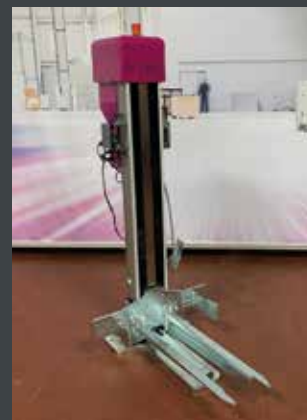
G8 Small and flexible up to 200 kg with electric linear unit, must be dowelled to the floor.
