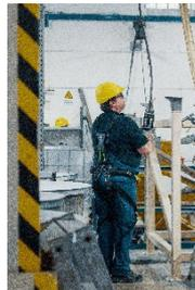
Efficient and Back-Friendly: Employees at GV Lacke use the BionicBack exoskeleton daily in intralogistics and production operations.
