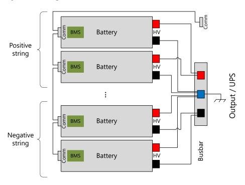
Example of system wiring with center tap. Other wiring configurations are possible, e.g. individual operation.
