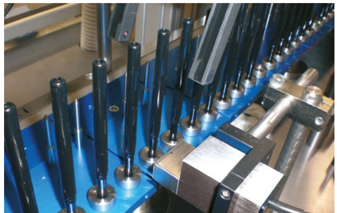
Precise application of oil on plastic parts
