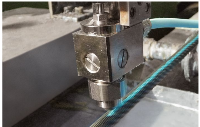
Color marking of wire cables
