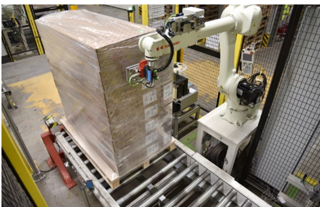
Robot labeling of pallets
