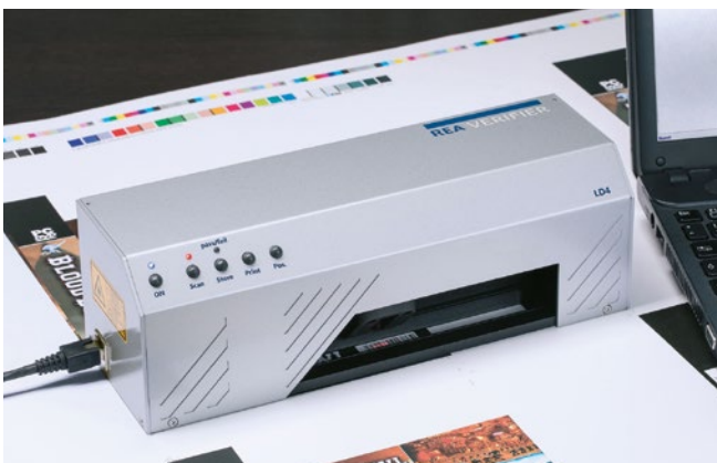
Measuring of barcodes on print sample sheets
