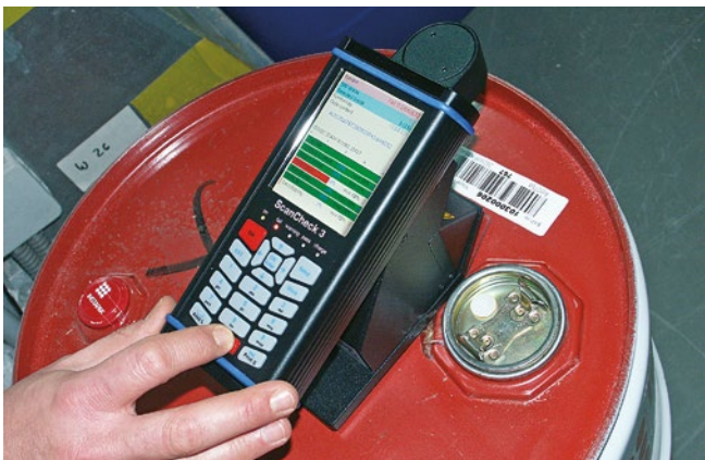
Verification of barcodes on metal drums
