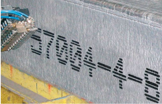
Marking of aluminum ingots
