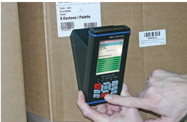
Flexible verification of barcodes on site
