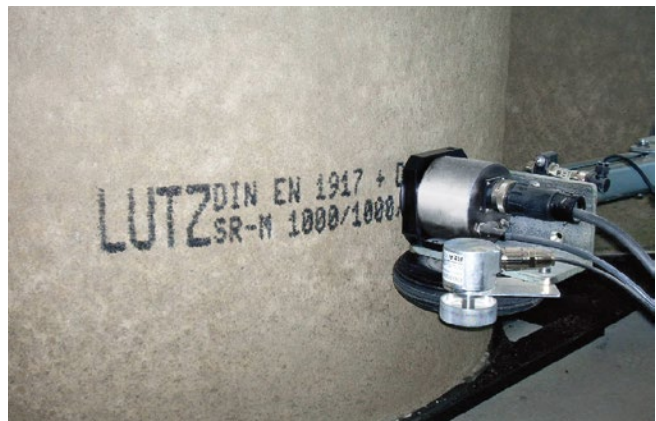
Marking of concrete pipes
