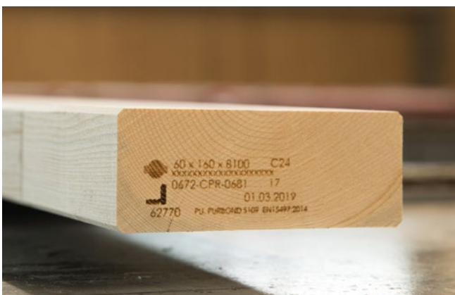
Wood marking with CO 2 laser
