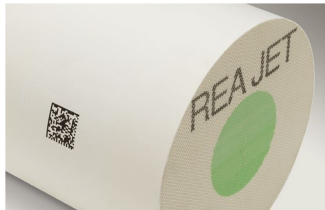
Marking of 2D codes on particle filters
