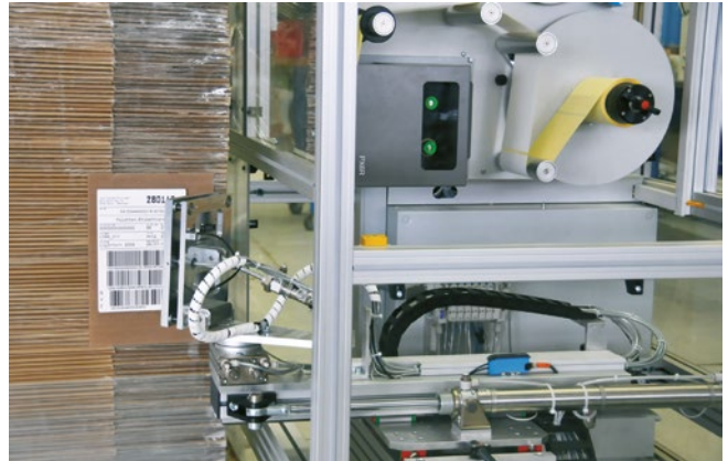
Pallet labeling (one stop for two sides)
