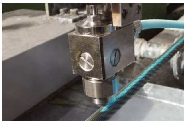
Color marking of wire cables
