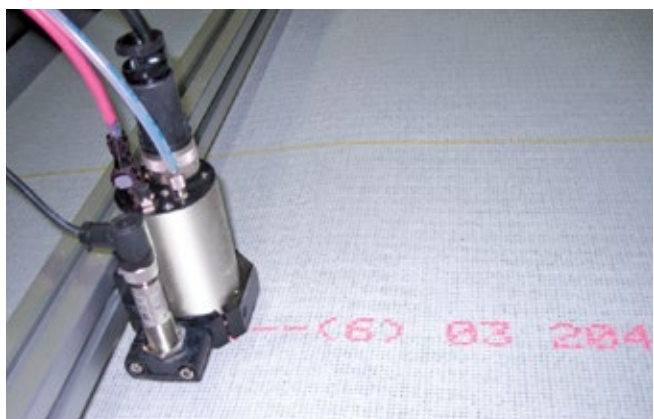
Coding and marking of sheeting materials
