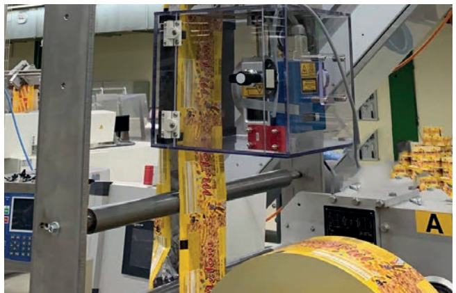
CL laser integrated into a packaging machine
