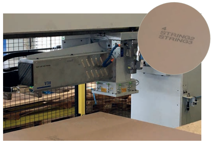
Laser system integrated into processing portal
