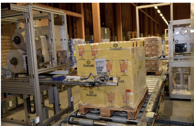
Pallet labeling at various heights
