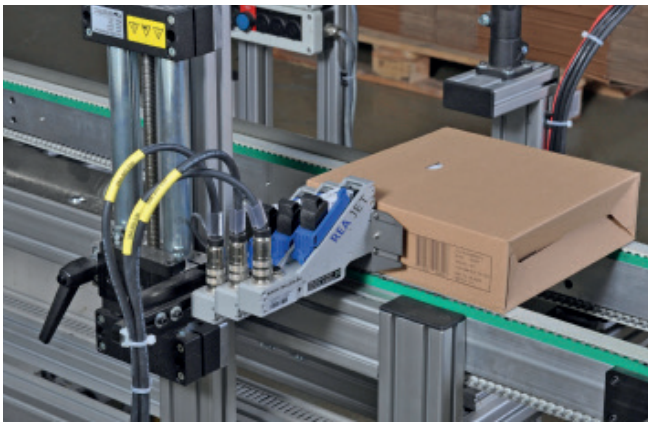
HR pro OEM integrated into a packaging line
