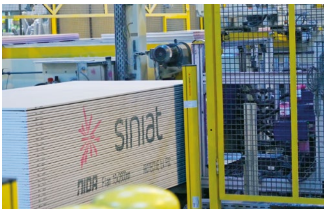
Marking of gypsum boards with large logos
