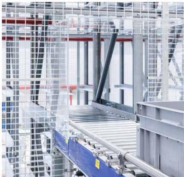
The compact design of the motor driven roller results in a high power density: A rated power of 57 W at 24 V or 115 W at 48 V ensures powerful drives.
