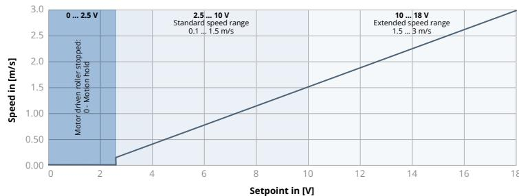
If the setpoint is below 2.5 V, the motor driven roller is held at a standstill via the "0-Motion Hold" function with rated torque.
