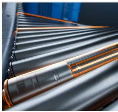
The motor driven rollers have a very high degree of efficiency. Their design is optimized to minimize friction losses in the drives. Savings of up to 30% compared to previous solutions are possible.
