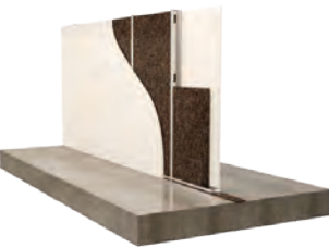
Internal partitions Metal-stud wall and slab discontinuity
