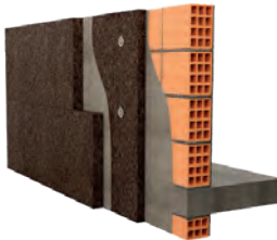
External walls External cladding over insulation - cork at sight
