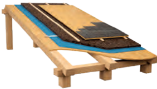
Roofs Pitched roof with above rafter insulation
