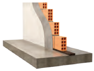
Internal partitions Masonry wall and slab discontinuity
