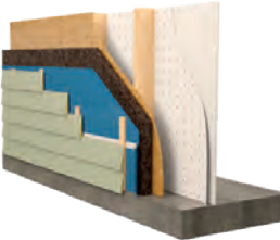
External walls Standard lap siding with exterior rigid insulation
