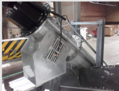
Free ejection with an clogging sensor
