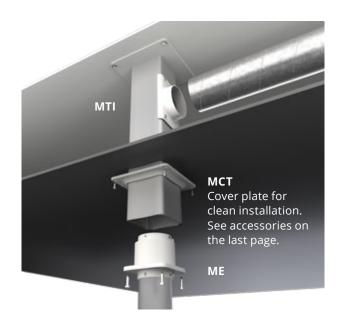
**ATEX (EX):** Aluminium and metal parts painted using special conductive paint (black), conductive polypropylene duct connection. Earth cable for safe grounding. Complies with the ATEX Directive 2014/34/EU category 2 gases and dust.
