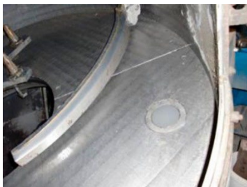
Microwave Moisture and Temperature Measuring System FL-MOBIMIC-SlimLine for Wireless Measured Value Transmission
