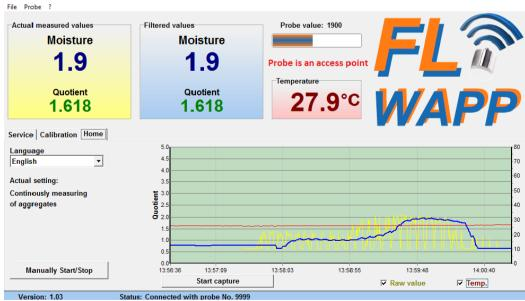
PC operating software for parameterisation, sensor calibration and measurement recording
