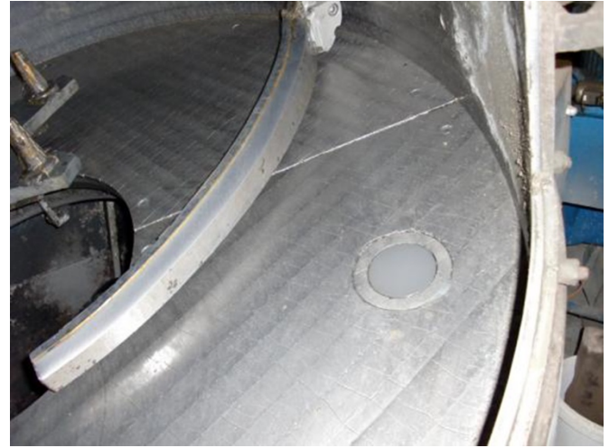
Sensor installation in a rotating mixer floor
