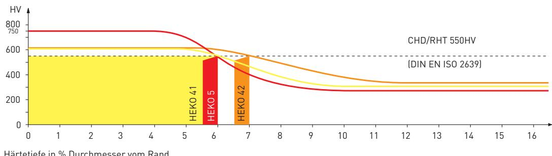
Hardening depth in % of diameter from the edge
