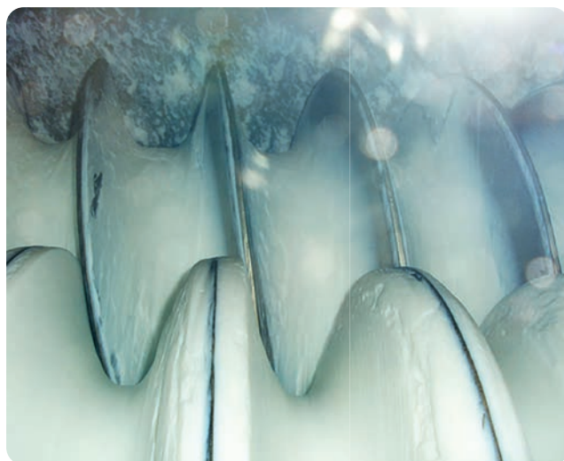
Product coating on screw flights
