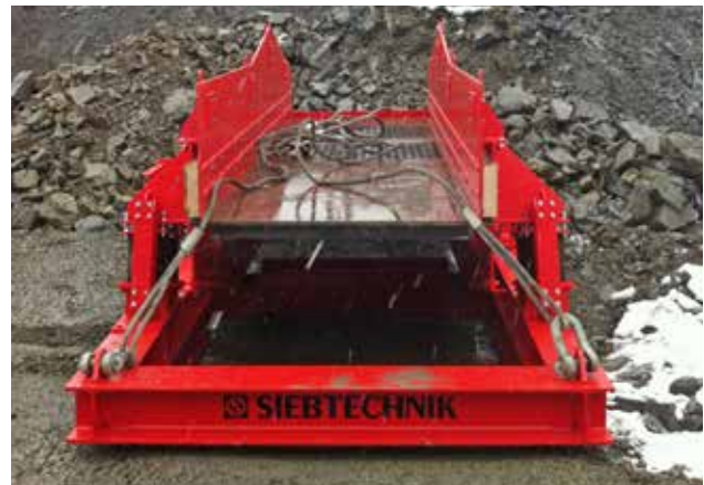
VS for a pre-screening system
