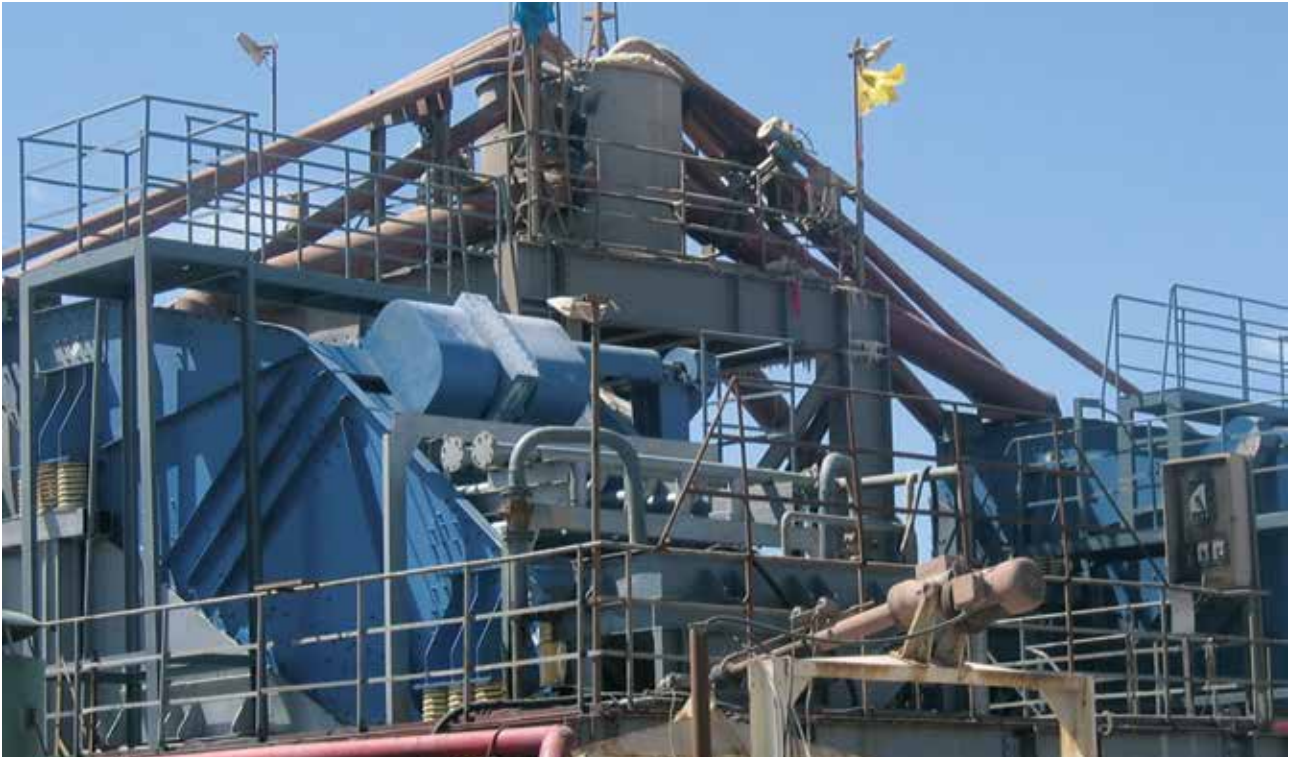
Geared screen, type BHG, banana screening machines for screening potassium salt in China
