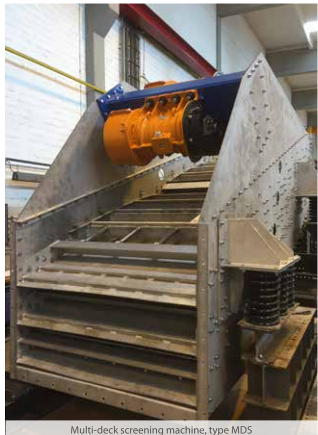
Multi-deck screening machine, type MDS, made from stainless steel
