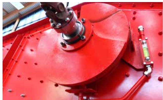
Unbalances with oil-level indication
