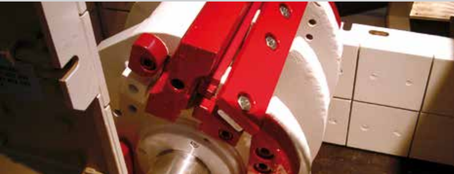
Impact bars for crushers
