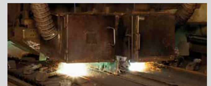
Production of VAUTID wear plates
