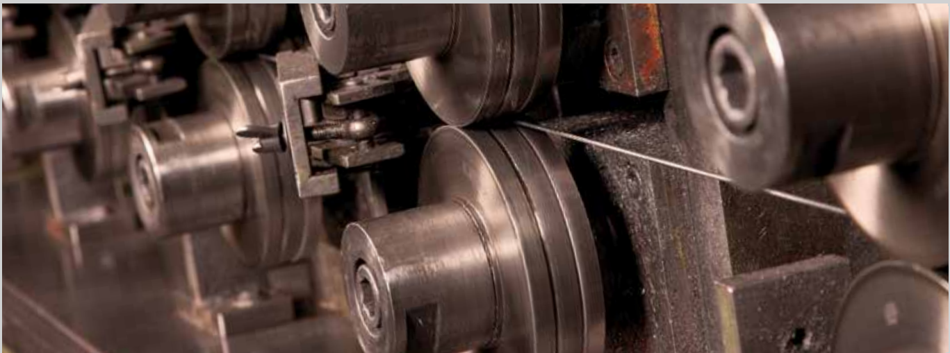
VAUTID tubular wire production
