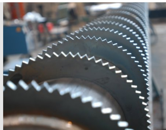
Screw shaft with toothed flights
