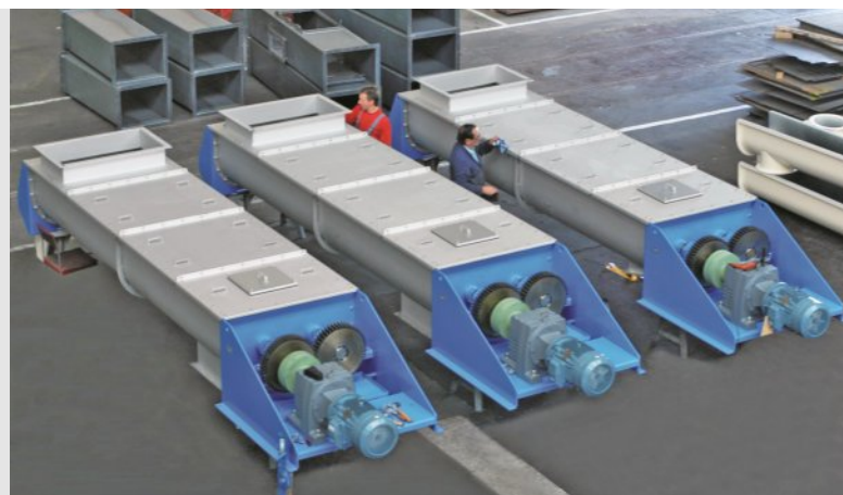
Factory-installed double mixing screw
