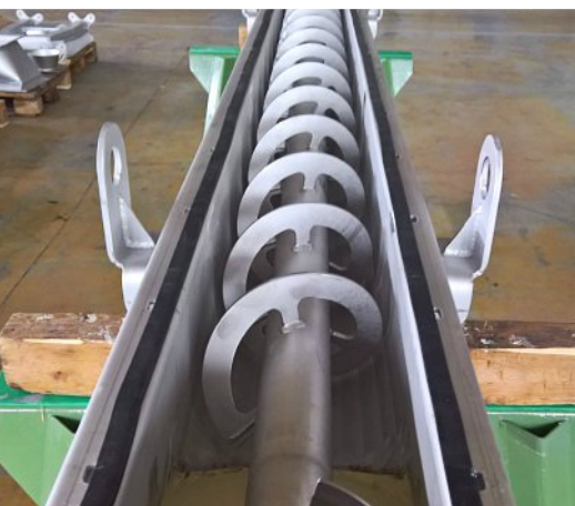
Screw conveyor with ribbon flights
