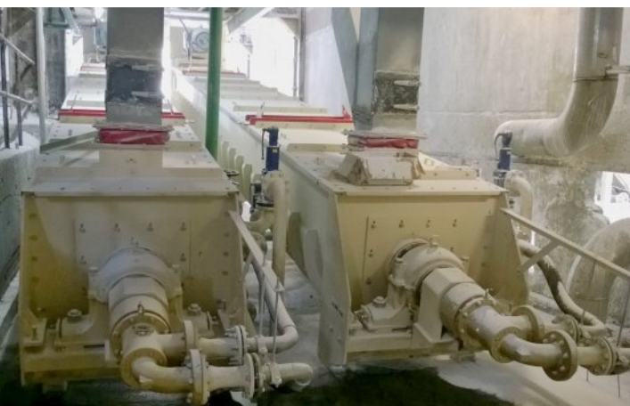
Cooling screw conveyors in operation
