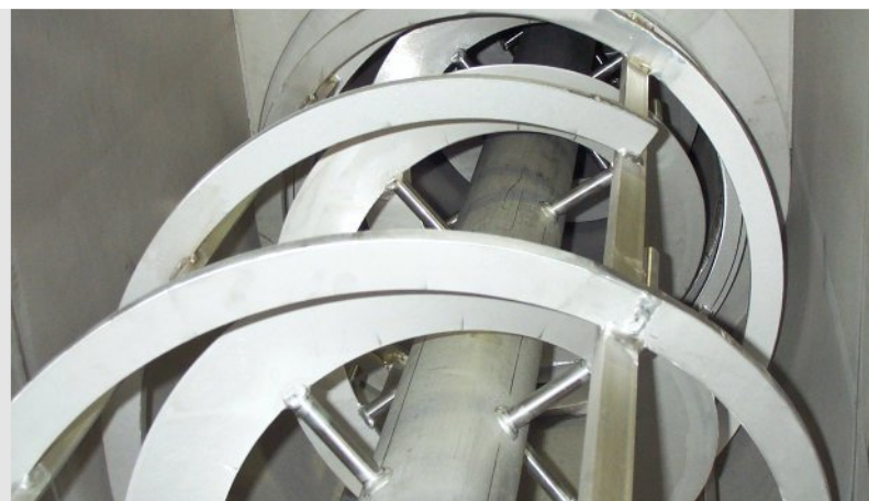
Shafts of a continuous flow mixer
