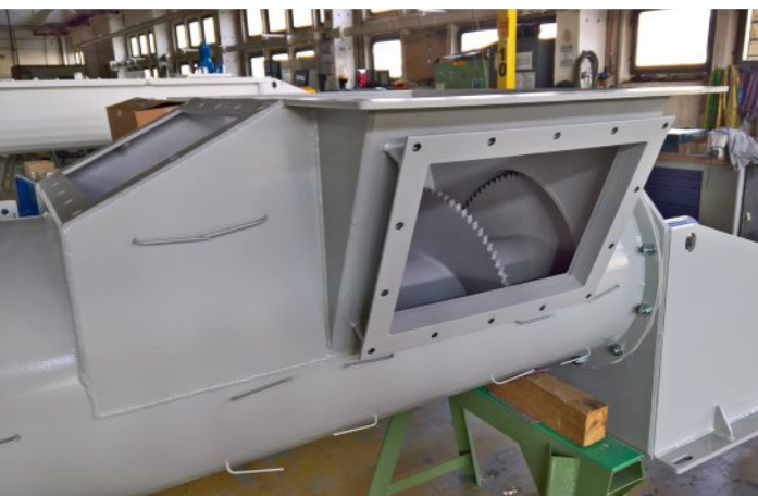
Tubular screw for the potash industry
