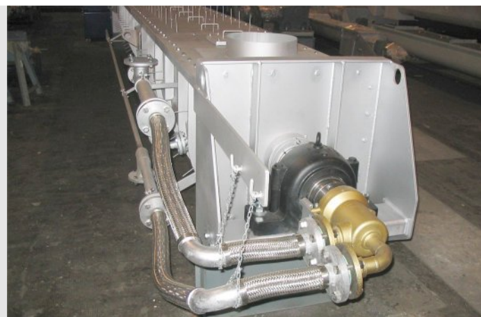
Rotary joint at the end bearing
