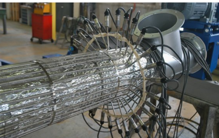
Workshop mounting of an electrical trace heating
