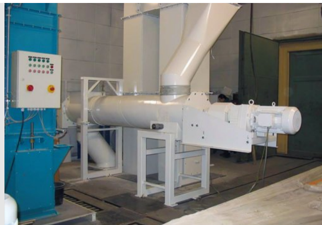
Weighing screw in our test stand
