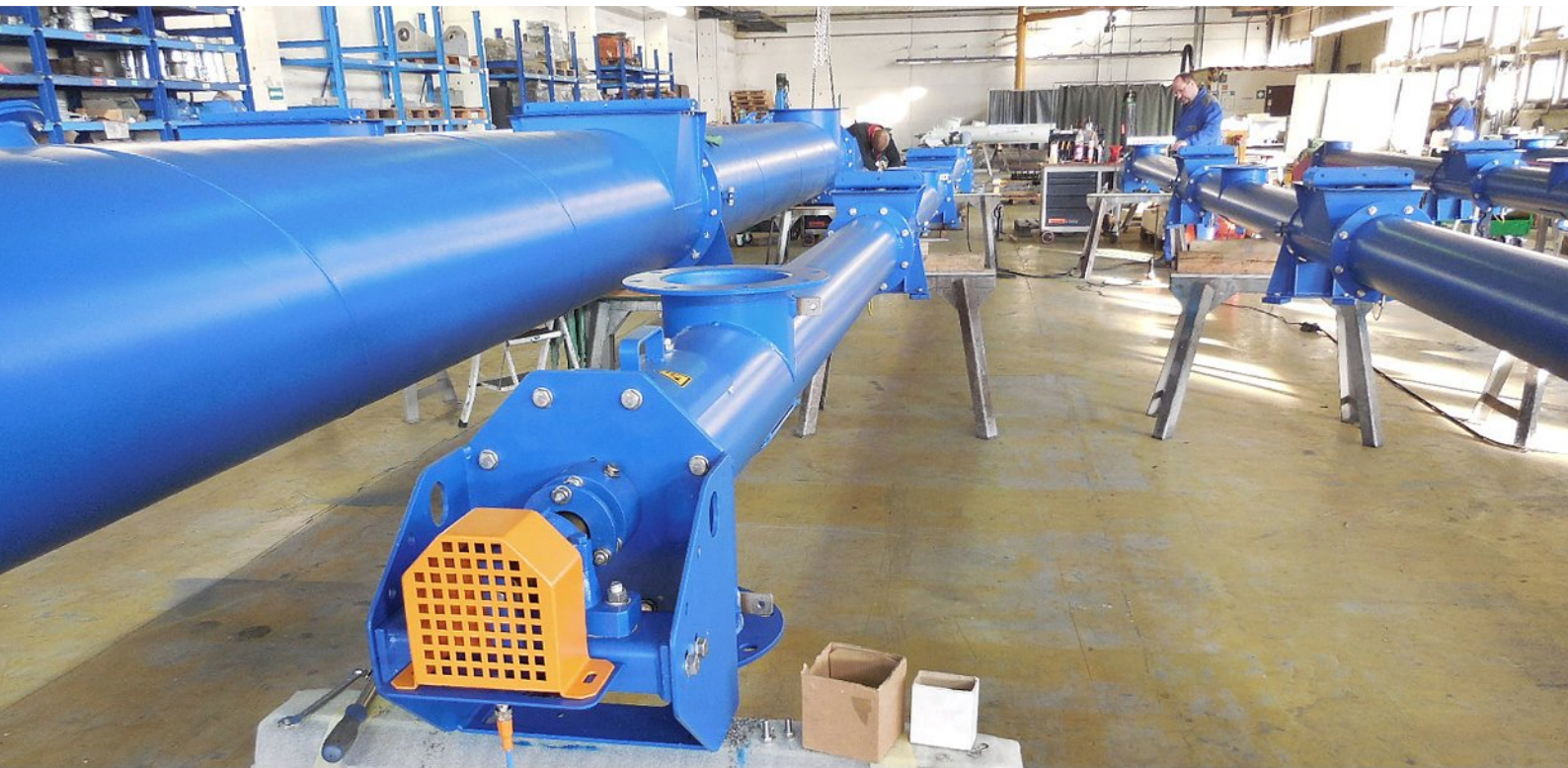
Final assembly of tubular screws
