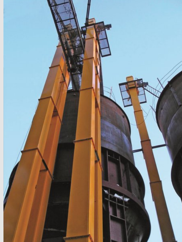
Bucket elevator for slate powder in Russia
