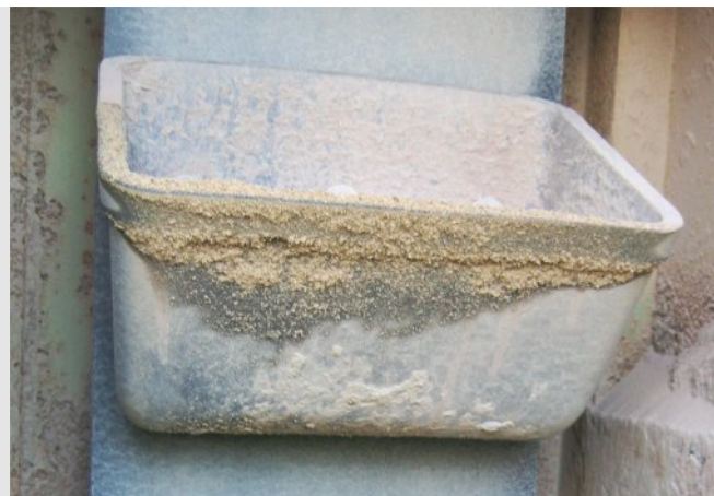
Cast polyamide buckets after a long term use for grit conveying
