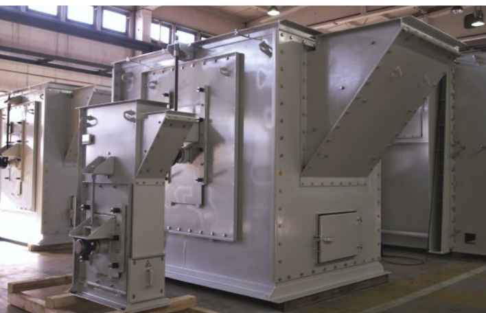
Bucket elevator boots in different sizes
