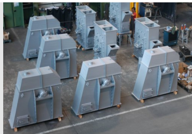
Final assembly of bucket elevator feet and heads
