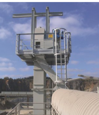
Bucket elevator head with maintenance stage
