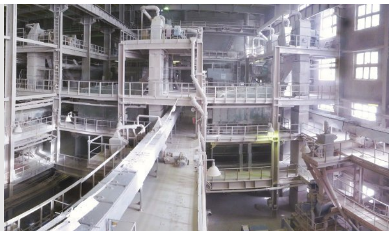
Bucket elevators in the potash industry
