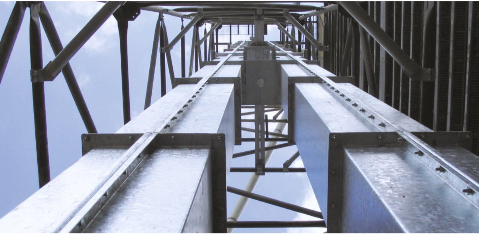
Grain bucket elevators in the steel-construction tower
