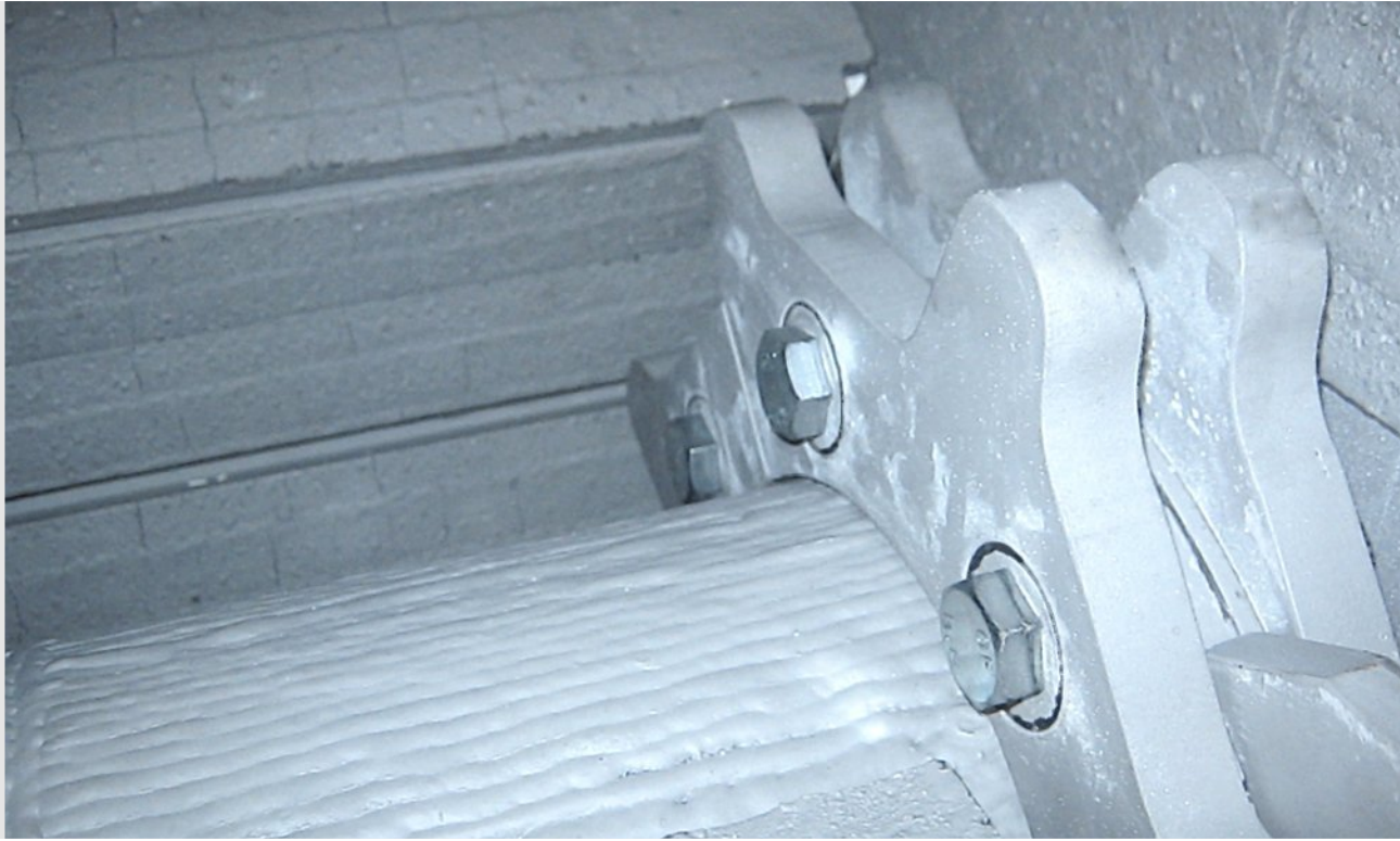
Material loop and shaft with wear protection
