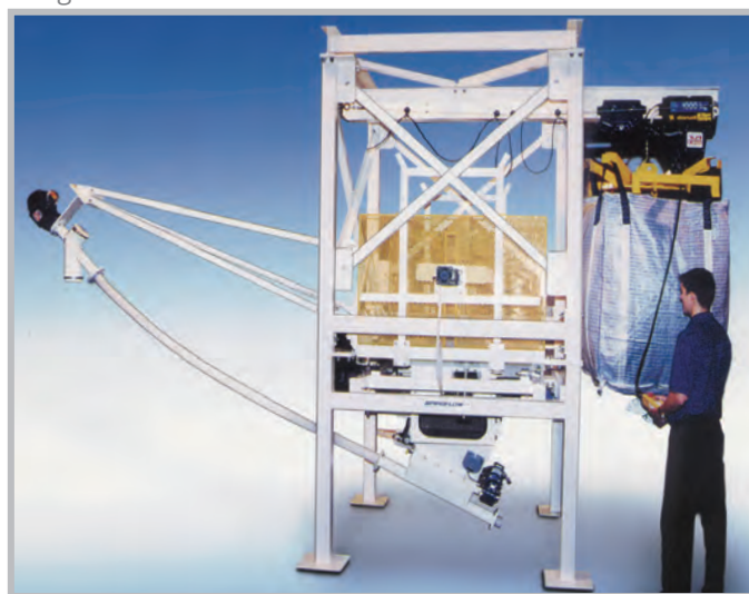
An optional low height hoist is available where headroom is restricted. The low height unit above has an overall height of under 11.5 ft / 3.5m & discharges 35 in. / 900mm bulk bags.
