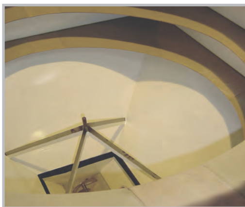
1. The T4 consists of a robust frame and discharge dish with a knife to pierce the base of the bag. A double membrane with dust extraction facility ensures total containment of dust emitted during the bag piercing operation.
