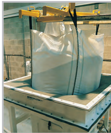
2. The double membrane ensures that the bag sits deep within the dish and no dust escapes during discharge.
