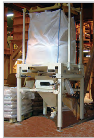
5. Bulk bag is loaded & ready to discharge
