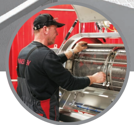
Centrifugal Sifter with Easy Access Wingdoors
