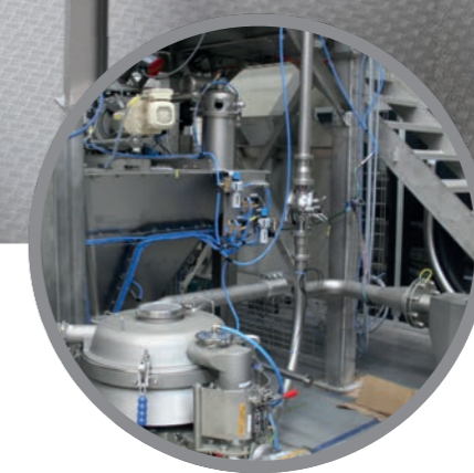
Inline Vibrating Sifter for pneumatic conveying
