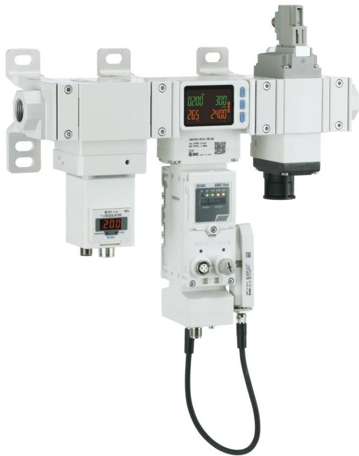
**Figure:** The new SMC Air Management System in 1/4 to 1-inch connection sizes comprised of a regulator, hub and shut-off valve offers potential savings in compressed air consumption of up to 62% thanks to the comprehensive monitoring of pressure, temperature and flow.
