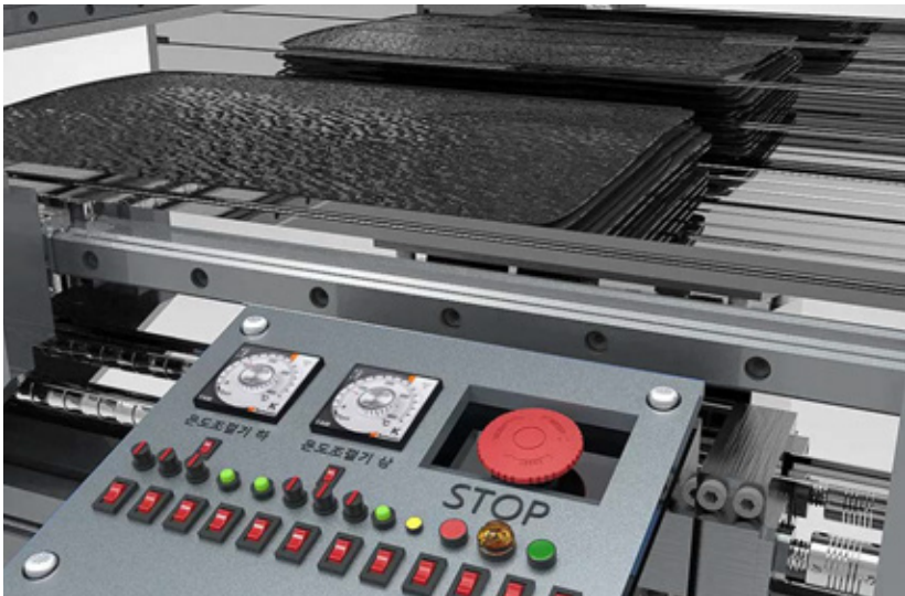
Plastic Bag Cutting Machines Temperature controllers are used to control the temperature of packaging material cutting machines.
