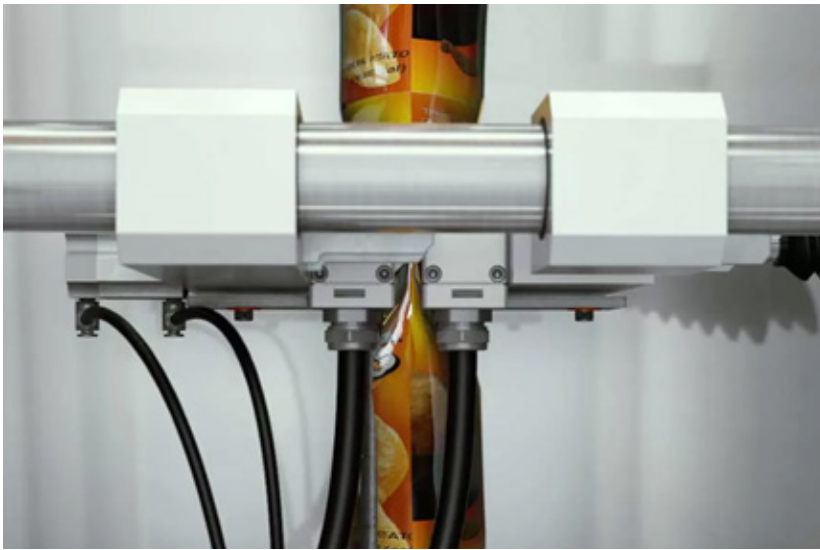
Chip Bag Filling, Sealing, and Cutting High performance PID temperature controllers are used to control heater temperature fast for chip bag filling and sealing.
