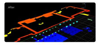
Intelligent denoising algorithms remove up to 99% of noise, ensuring reliable and stable inspection in challenging scenarios.
