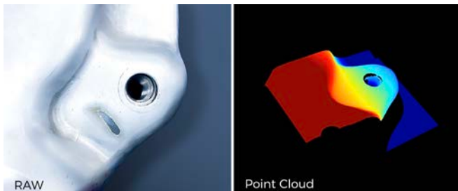
Threaded hole Mech-Eye UHP-140-GL @ 0.3 m, point cloud rendered by height
