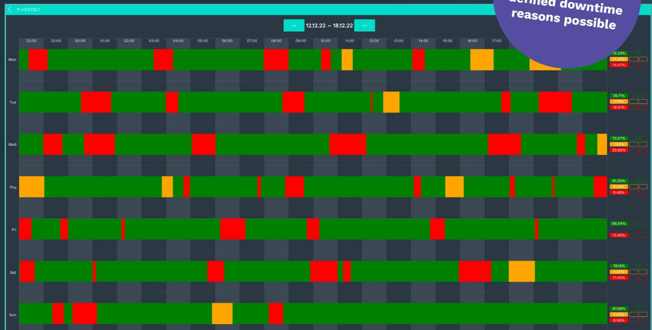
Exemplary display of a milling machine with downtimes and productive times including piece counting
