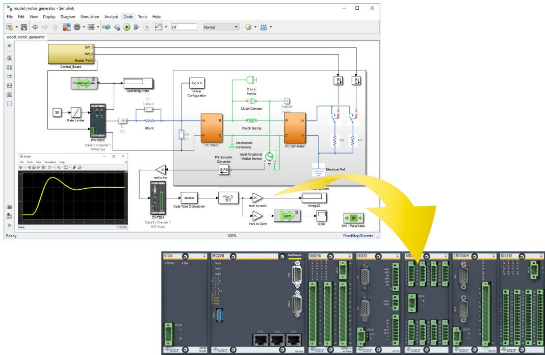
▼ *Simulation – Solution development on the computer model and direct download to the M200 Controller System*
