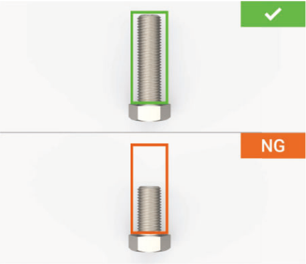
Length Inspects the captured image in reference to the length set by the user between two edges of the registered image.
