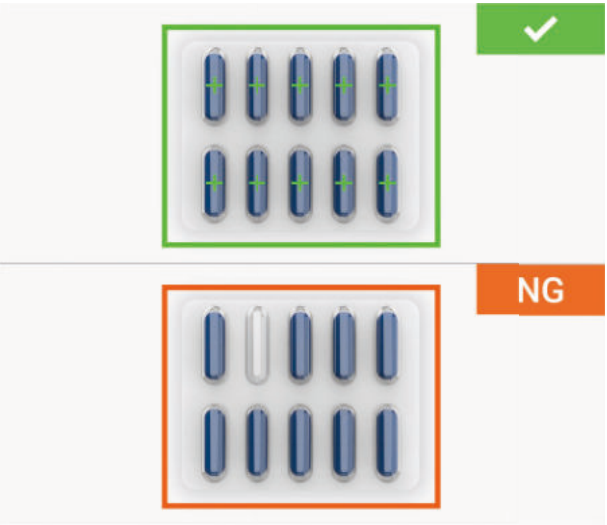
Object of Color Counting Inspects the number of specific colored objects in the captured image's ROI in reference to the registered number of colored objects in the registered image's ROI.
