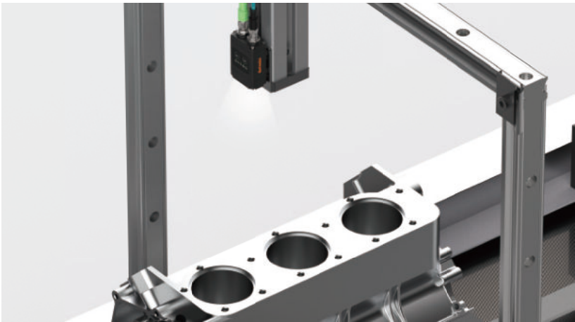
9-4. Automobile Parts Manufacturing Line Visions sensors are used to identify the diameter of holes in car engine blocks during manufacturing.
