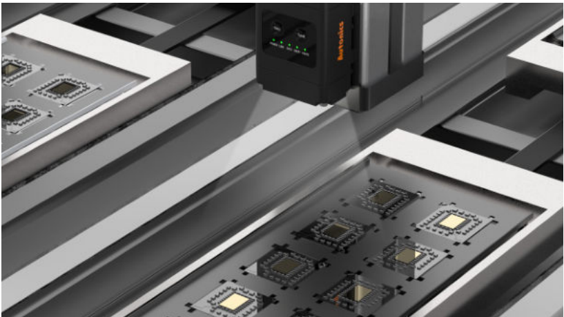
3-2. Semiconductor Parts Transfer Line Vision sensors are used to identify the presence or absence of parts for defects during semiconductor transfer lines.
