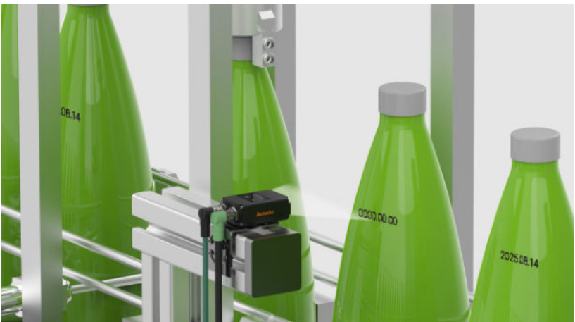
7-2. Beverage Containers Packaging Line Visions sensors are used to identify the presence of expiration date printing on packages.
