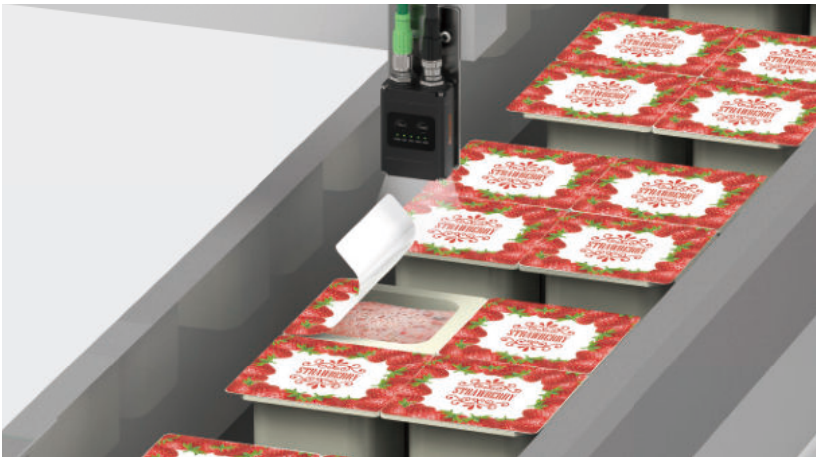
7-1. Containers Transfer Line Visions sensors are used to identify sealing status of food containers on conveyor belts.
