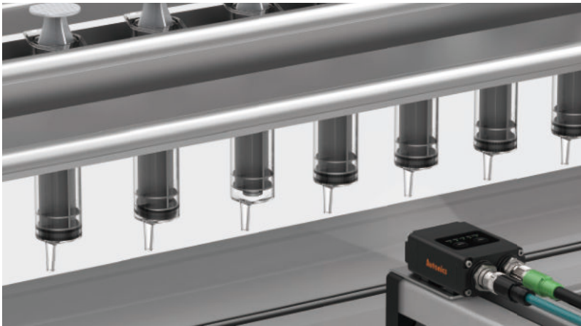
2-1. Syringes Assembly Line Visions sensors are used to identify presence, absence, or defects of rubber packing in syringes during manufacturing.
