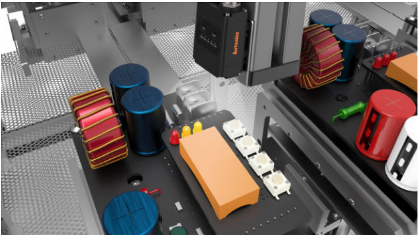
3-1. PCB Transfer Line Color type vision sensors are used to identify colors of diodes and capacitors on PCB boards during manufacturing process.
