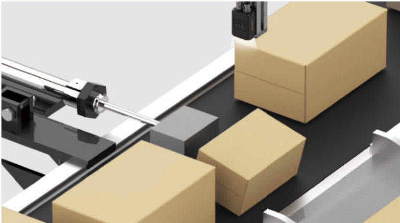
6-1. Shipping Transfer Line Visions sensors are used to identify box sizes on shipping conveyor belts.
