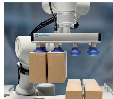
*Examples of HVGEE electric palletizing suction devices
