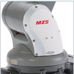
Stopper cover for reducing clamping risk
