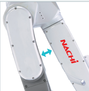
Offset arm shape for reducing clamping risk
