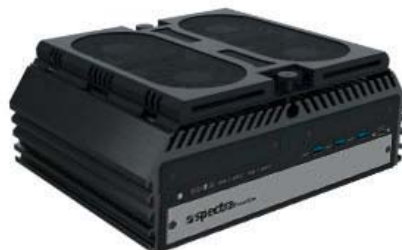
External fan accelerates heat dissipation
