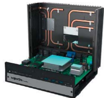
Independent cooling for CPU & GPU
