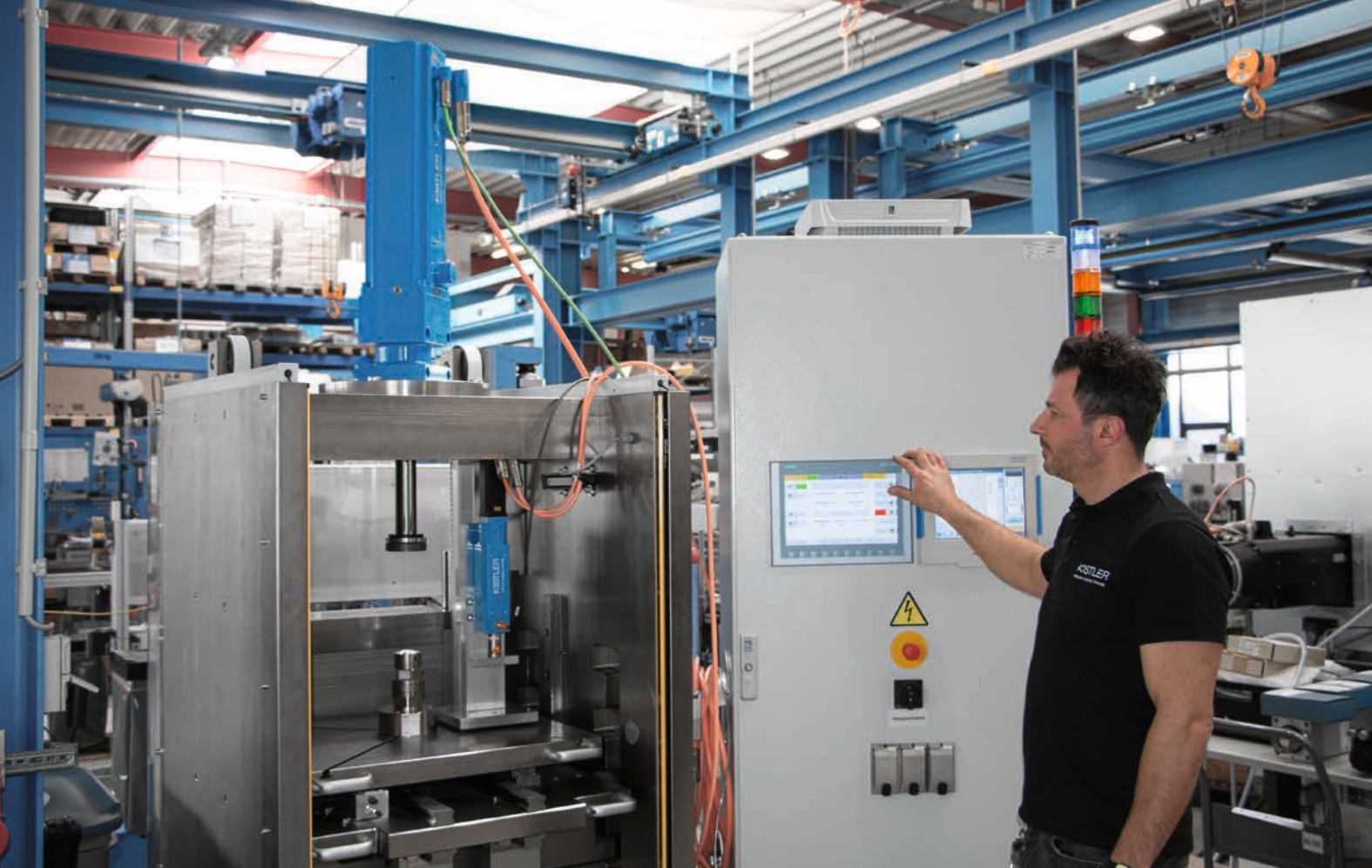
The Kistler test workstation comprising the frame, NC joining module, control cabinet with measurement technology, control and data acquisition unit
