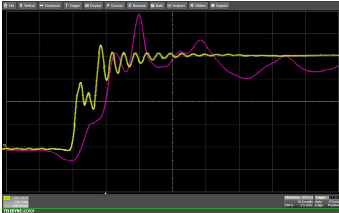
FIGURE 6. Comparison of Waveforms on a LeCroy Oscilloscope with IsoVu Waveform Overlaid.
