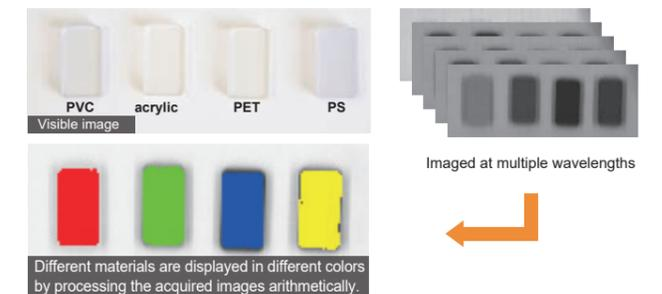
Different materials are displayed in different colors by processing the acquired images arithmetically.
